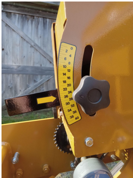
Figure C - Knob to adjust gear setting
