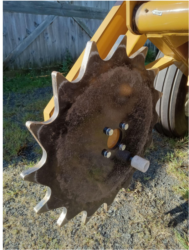
Figure G - Drive wheel. 130 turns = 1/10 acre
