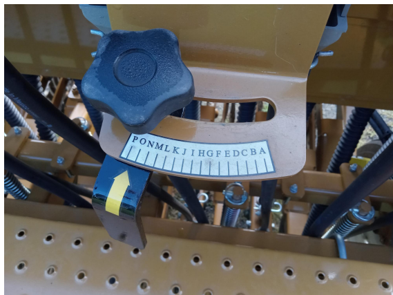
Figure E - Knob to adjust seeding rate for small hopper
